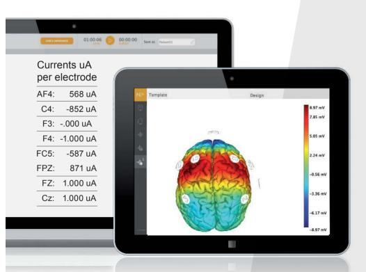
Wireless & Hybrid Device tDCS, tACS, tRNS or user-defined waveform Multi-electrodes Real-time EEG during tCS Sham, active sham and double-blind modes
